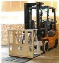
Push/Pull attachment grips and pulls the sheet with goods on it back onto the forks
