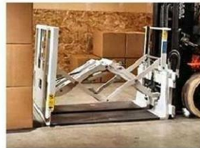
Push/Pull attachment grips and pulls the sheet with goods on it back onto the forks
