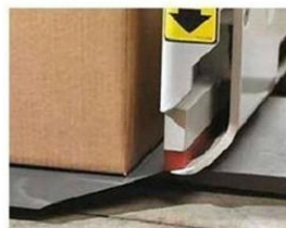
The Slip-Sheet is gripped by a special rubber clamp preventing any damage to the sheet
